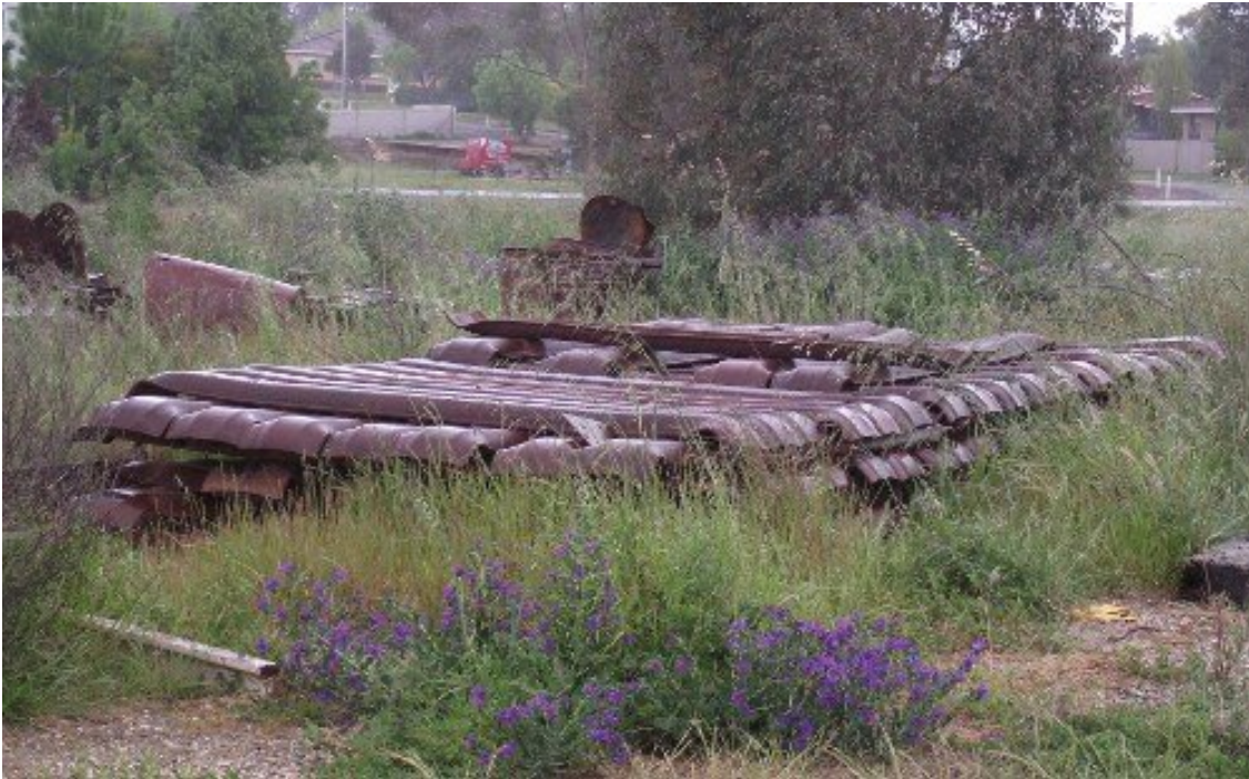
Above: Steel sleepers at Wahgunyah
